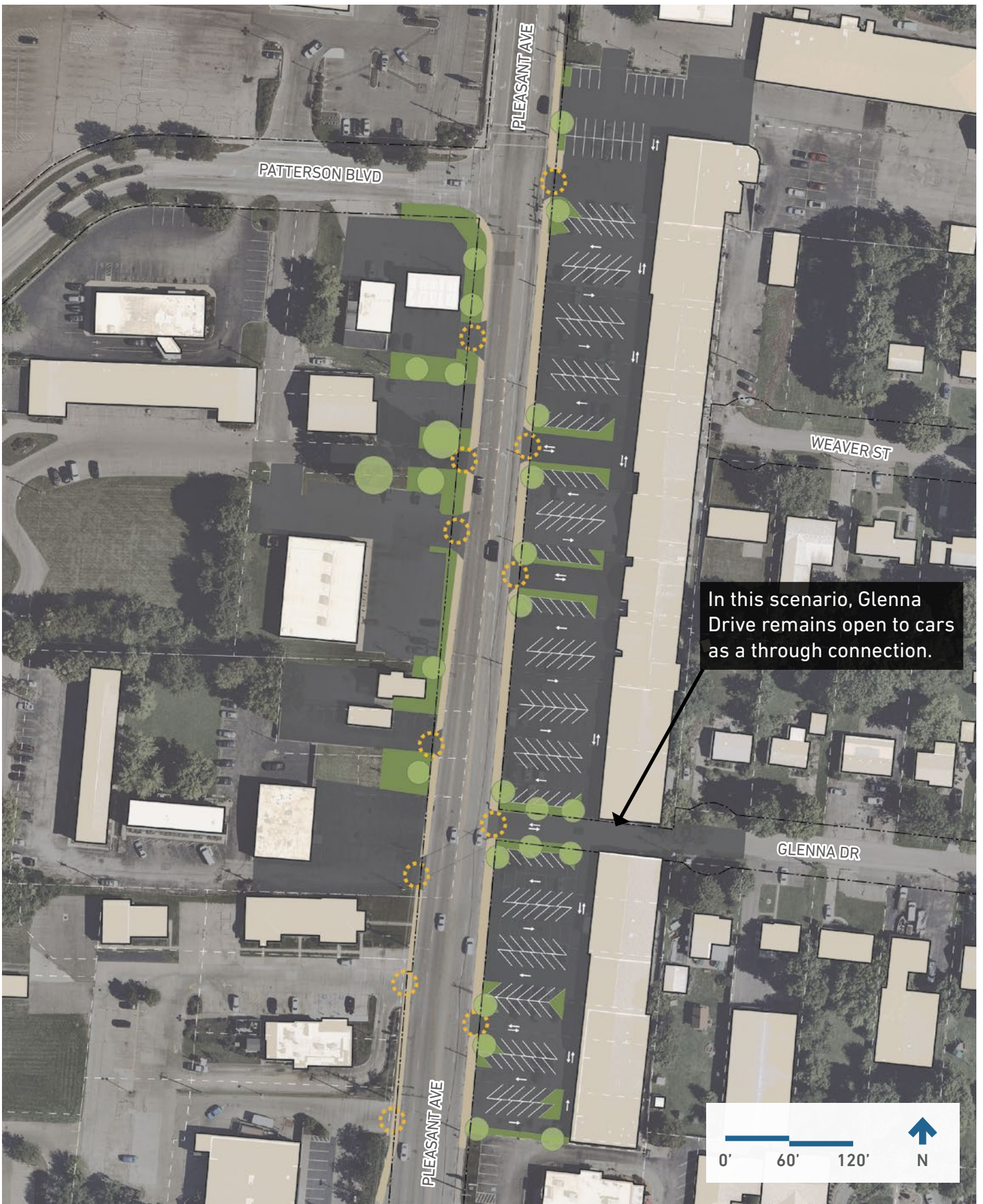
Figure 10: Scenario 2: Angeled Parking with Access Management
