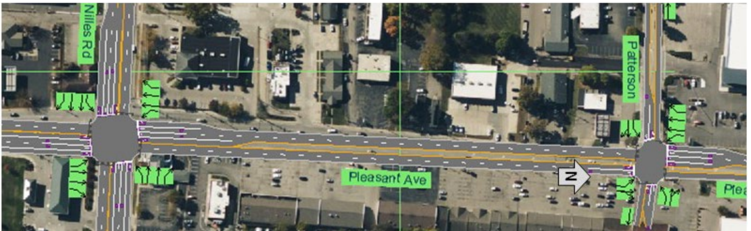
Figure 16: Existing Lane Configuration - Pleasant Avenue
